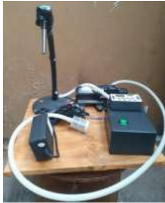
Gambar 5 Alat pengisian cairan kedalam botol low budget
